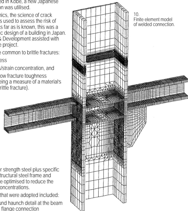
10. Finite element model of welded connection.
