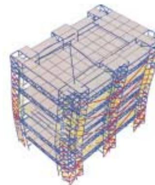
8. LS-DYNA 3D model showing OICC's seismic performance.
